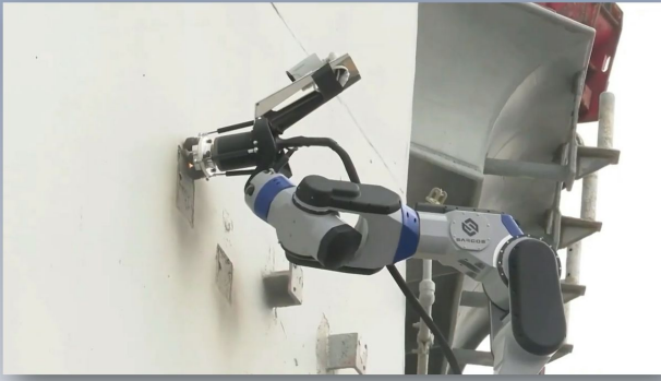
Plasma / laser ablation to remove material from the side of the ship
